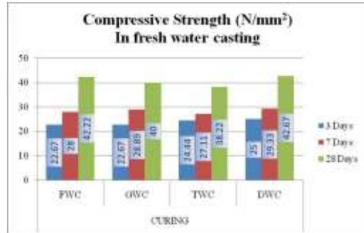
Fig 16: Concrete Compressive strength in FWC
