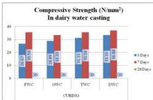
Fig 15: Concrete Compressive strength in DWC
