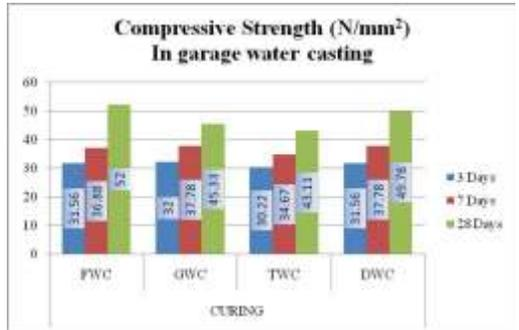
Fig 13: Concrete Compressive strength in GWC
