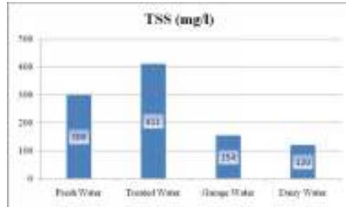
Fig 6: Comparison of Total suspended solids
