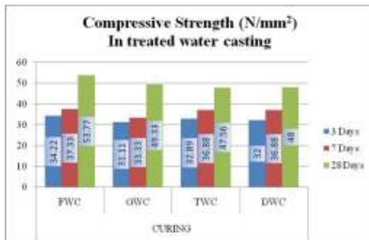
Fig 14: Concrete Compressive strength in TWC
