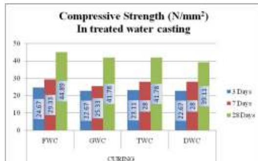
Fig 17: Concrete Compressive strength in TWC
