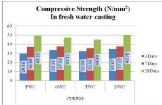
Fig12: Concrete Compressive strength in FWC
