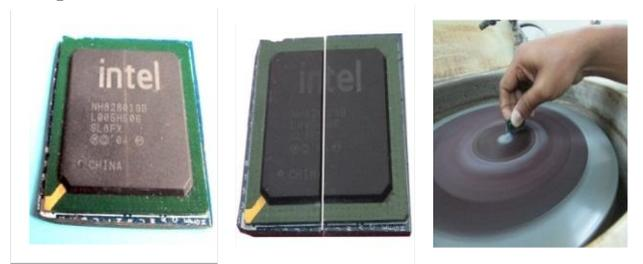
Figure 3 – Processing of the PBGA component for the tensile testing of BT and for Microscopic analysis.
