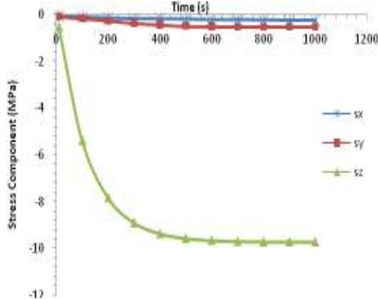
Fig. 5. Plot of thermal stress values with time for element 2258
