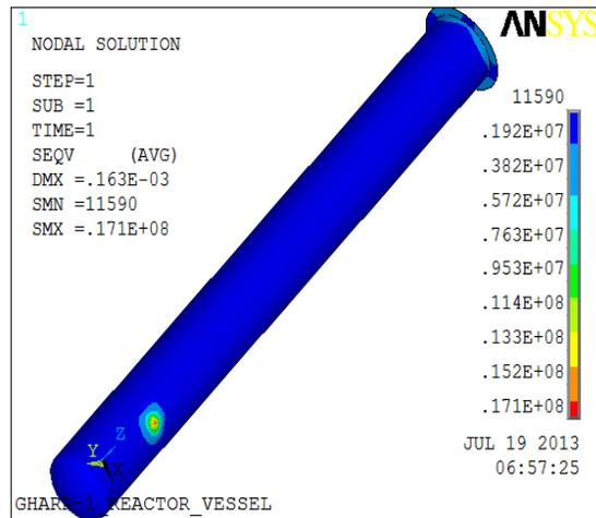
Fig. 7. Effective stress distributions at steady state
