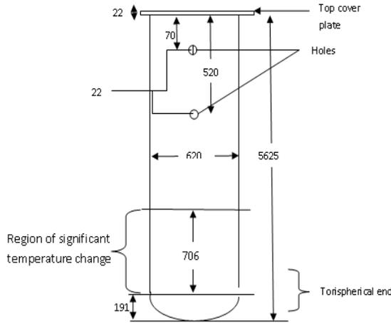
Fig. 2. Longitudinal section of GHARR-1 showing region of significant temperature change
