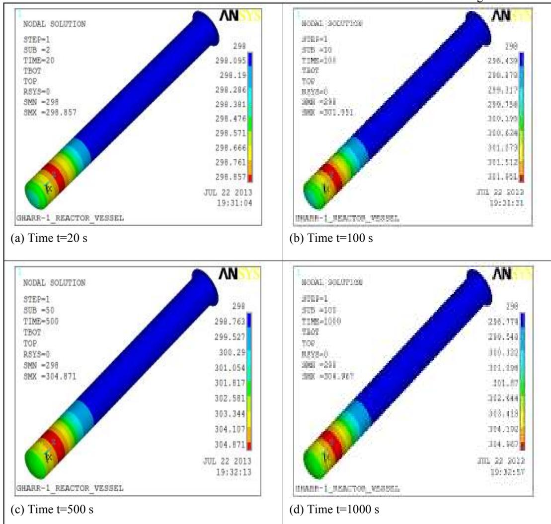
Fig. 4. Plot of temperature distribution for different time-steps
