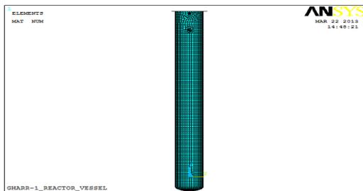
Fig. 1. Finite element model of the GHARR-1 Vessel
