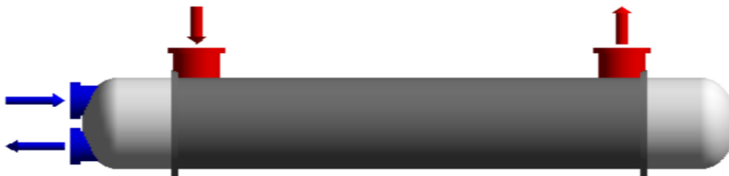
Fig. 1. A layout and hot gas and cold coolant passage of shell and tube heat exchanger
