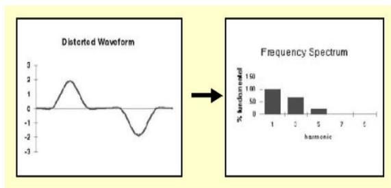
Figure. 1 Relationship of Distorted Waveform with Frequency Spectrum
