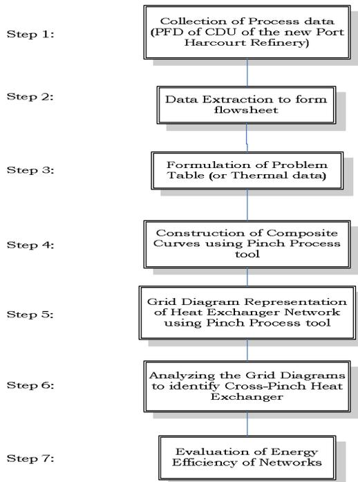
Figure 4: Flowchart for Pinch Analysis
