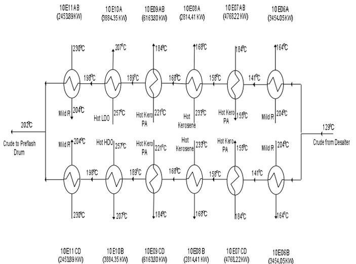
Figure 2: Heat exchangers configuration showing all streams in HEN-2
