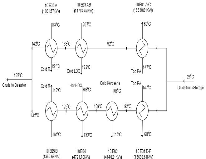
Figure 1: Heat exchangers configuration showing all streams in HEN-1
