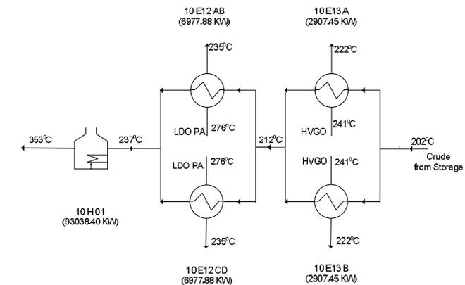
Figure 3: Heat exchangers configuration showing all streams in HEN-3
