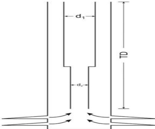
Fig.2 Dual Completion Tapered Tubing
