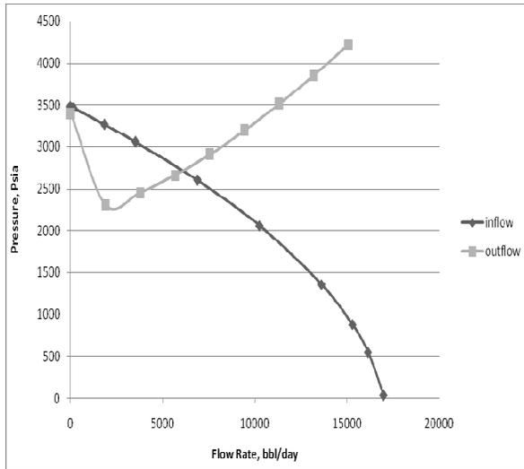
Fig. 10 Nodal Analysis of 2.992 and 3.340 in. tubing
