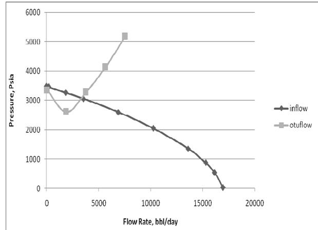
Fig.8 Nodal Analysis of 1.995 and 2.441 in. tubing
