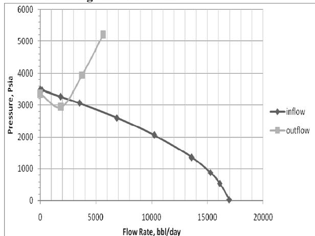
Fig.5 Nodal Analysis of 2.441 in. tubing
