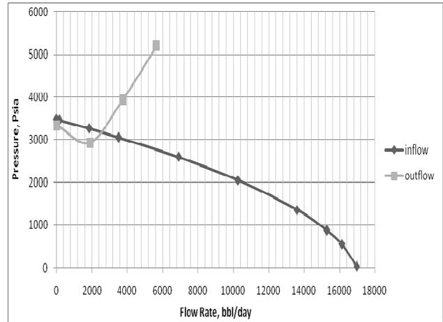
Fig. 4 Nodal Analysis of 1.995 in. tubing
