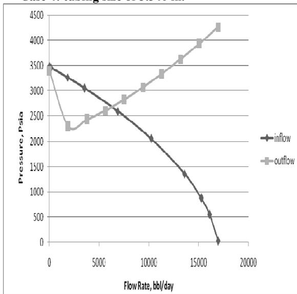
Fig.7 Nodal Analysis of 3.340 in. tubing
