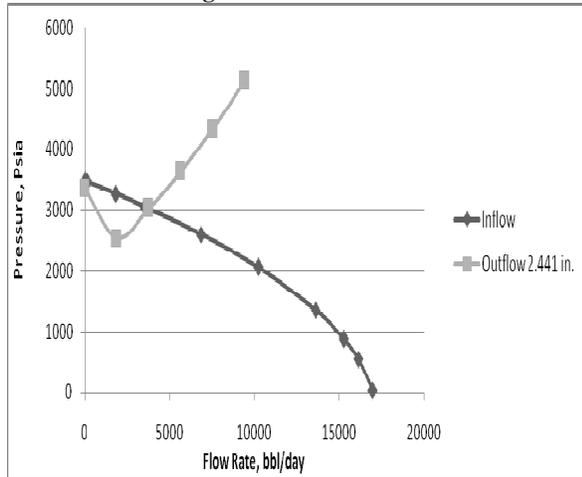
Fig.6 Nodal Analysis of 2.992 in. tubing
