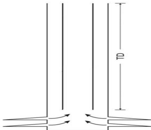
Fig.1 Conventional Tubing Completion
