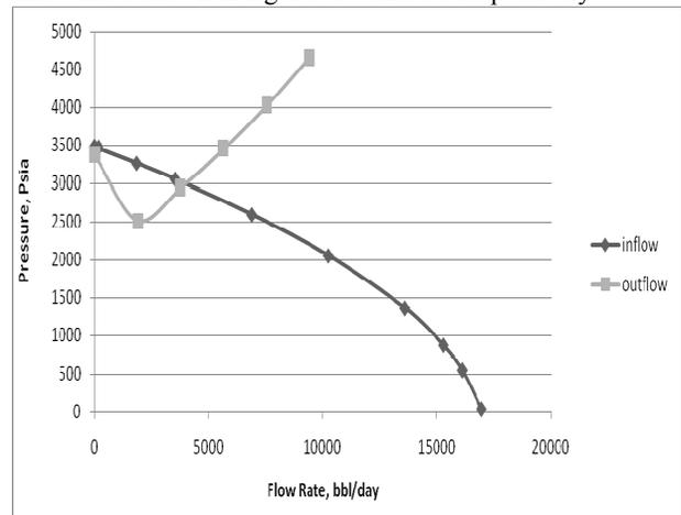
Fig.9 Nodal Analysis of 2.441 and 2.992 in. tubing
