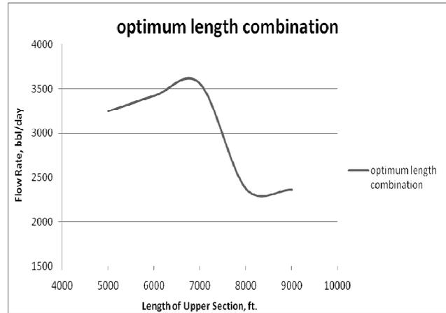
Fig. 11 Optimum Length Combination of 1.995/2.441 in.
