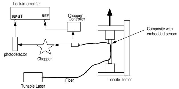
Figure 2: The Experimental Set-Up
