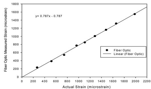
Figure 3. Fiber Optic Measured Strain versus Actual Strain
