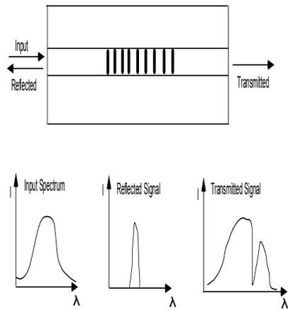
Figure 1: Reflected and transmitted Bragg grating signal with a broadband source
