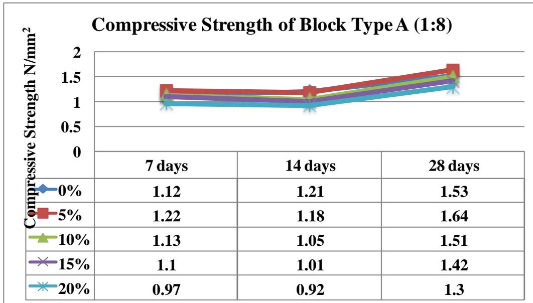
Figure 2: Compressive Strength of Sandcrete Block (1:8)
