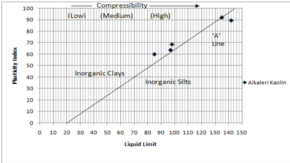
Figure 1: Casagrande Plastic Index-Liquid Limit Classification of Alkaleri Kaolin
