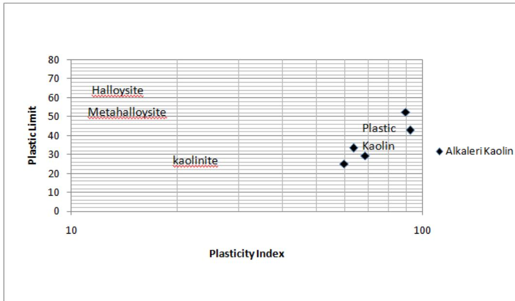
Figure 2: Plastic Limit-Plastic Index Classification of Alkaleri Kaolin.
