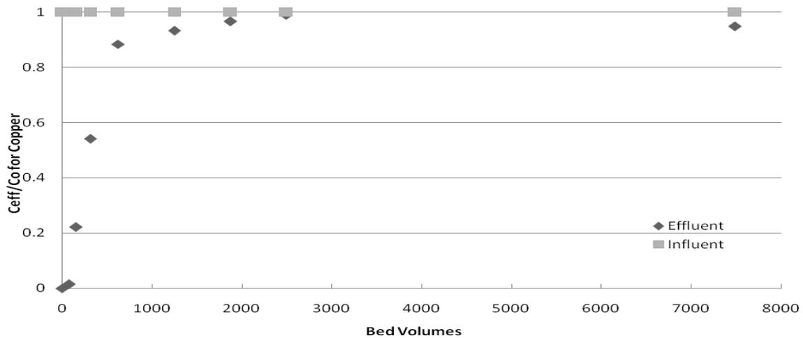
Figure 6: Breakthrough Curve of Cu versus Bed Volumes
