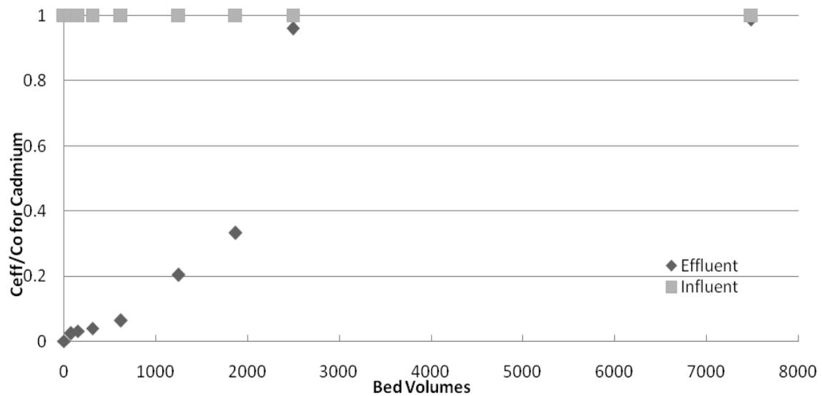
Figure 7: Breakthrough Curve of Cd versus Bed Volumes
