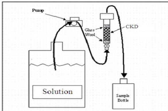
Figure 1: The Column Experiment Setup
