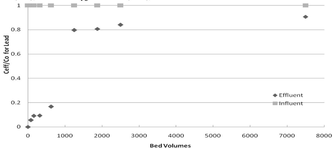
Figure 5: Breakthrough Curve of Pb versus Bed volumes
