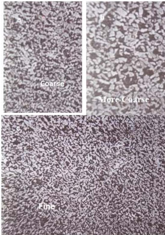
Figure 1: Microstructure of Aluminium cast using (a) River Niger Mould (coarse) (b) Ochadamu Sand Mould (more coarse) and (c) Uwowo Sand Mould (fine). Nital etched x100.
